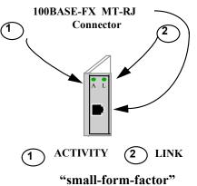
ACTIVITY (A) and LINK (L) LEDs to indicate proper connectivity with the remote device. It has the same "100Mb FX" lettering on the faceplate. Note that the other end of the fiber cable may have a different connector, not necessarily an MT-RJ type.
